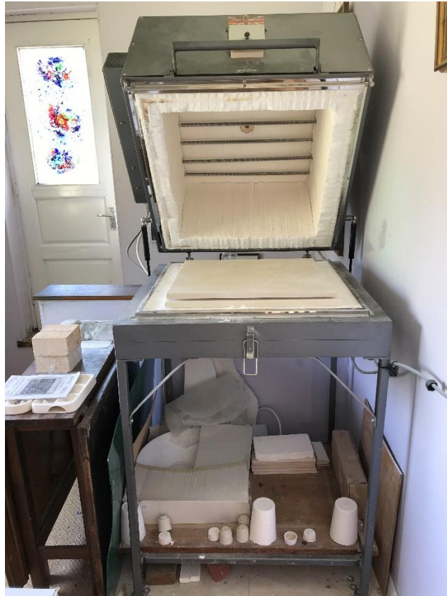
1) Northern Kilns FB46. 450mm x 450mm x 230mm high. Glass kiln
